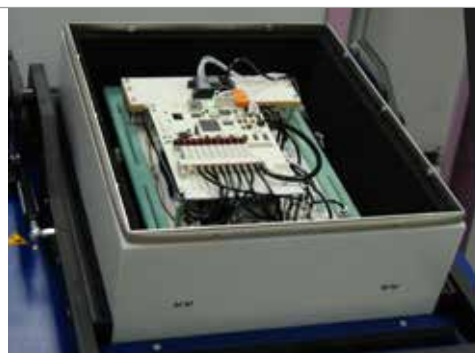
Picture showing the YAV90PNF, implemented inside an RF fixture
