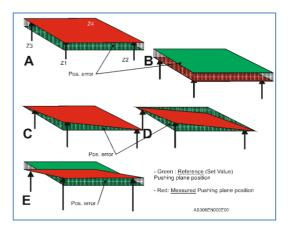
With the AS206 set you get a quick measurement of the precision and accuracy values of the pushing system on the automatic test platforms.
