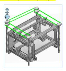
The AS206 system works with four position sensors for the four corners of the fixture and two laser beams, mounted diagonally, pointing to the center of the CCD cameras.
